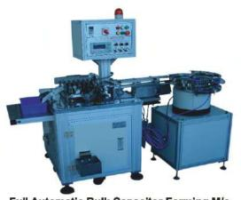
Full Automatic Bulk Capacitor Forming M/c
