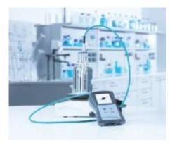
The ZESTRON<sup>®</sup> EYE Mobile is the ideal tool to monitor the cleaning agent concentration of several pcb and stencil cleaning machines with only one device. Configure preset profiles for individual locations using the intuitive software menu allowing even untrained operators to make fast, precise concentration measurements.
