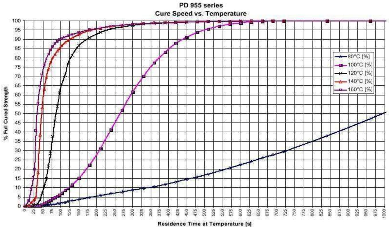
Adhesion is sufficient at 85 % full cured strength.
