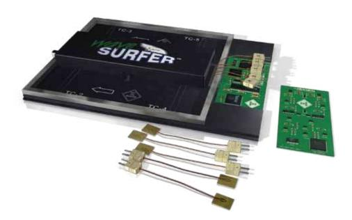
Check your wave soldering proce and finetune your machine for optimum performance with the KIC Wave Surfer $^{TM}$ .
