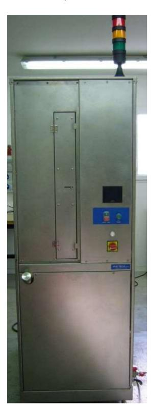
Specially designed to provide high cleaning performance, the stencil is introduced into the loading cell of the equipment and automatically immersed in the upright position and submitted to the superior cleaning performance of perpendicular ultrasound and is perfectly cleaned in just a few minutes.
